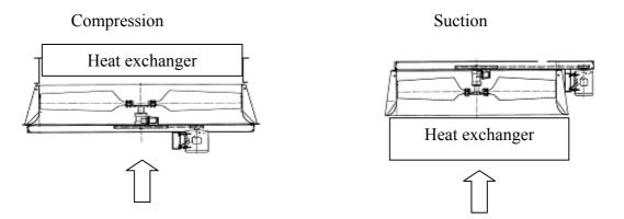
With the compression method, the air first passes the ventilator, which then pushes (compresses) the air through the heat exchanger.
